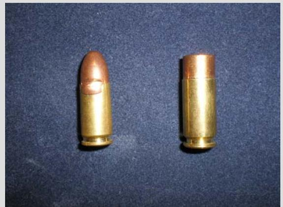
**The cartridge on the left has bullet jacket material overlapping the mouth of the cartridge case. This round would go into a magazine just fine, but would not chamber in your pistol. The round on the right is a factory loaded cartridge with the bullet seated backwards. Always check ammo you will be carrying for self defense.**
