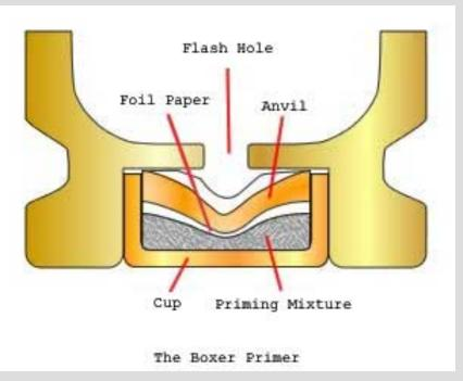
The primer contains a pellet of explosive, that is detonated by the impact of the firing pin. This pellet must be intact for the primer to fire.
